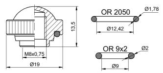
For coil series 3 and 4 (solenoid valves 3/2NC)
